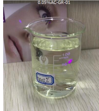
● 0.05% AC-GR-01 solution Blue light is almost completely absorbed
